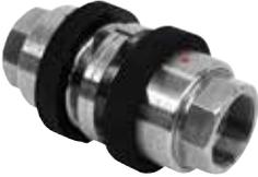
The shear pin Breakaway is designed to function with pull forces that are designed to pull at an angle of 10 degrees or greater from the center line of the Breakaway. The shear pins separate at a pre-designed force closing the valves. These type Breakaways are used on piping systems to connect hoses and loading arms as protection to prevent high forces that may break the loading arm or hose. It also protects the piping system from damaging pull forces.
