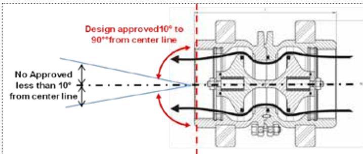
19. **Cable Breakaway** - When using a Breakaway that is triggered by cable pull, this design can operate with a pull angle from  $0^\circ$  to  $90^\circ$ . **The cable length must be shorter than the hose.**
