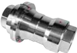
This shear pin Breakaway type is designed to function with straight pull forces commonly found in hose strings. The shear pins separate at a pre-designed force (designed based on the type hose used) closing the valves. It is only designed to be used on straight pull hose applications.
